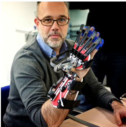
Figure 1. SCRIPT1 passive hand/wrist orthosis
